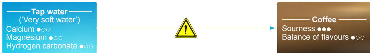
Figure 19: 'Very soft water' contains hardly any calcium and magnesium ions and hydrogen carbonate. This can result in coffee with extreme sourness and an unbalanced flavour.
