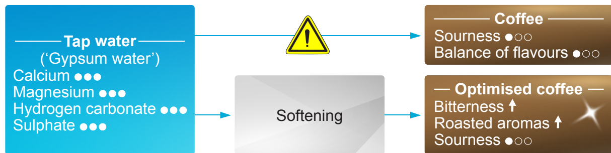
Figure 13: The only way to effectively protect coffee machines from permanent hardness is to soften it first. This results in a coffee taste with (unchanged) low sourness and pronounced bitterness and roasted aromas.
