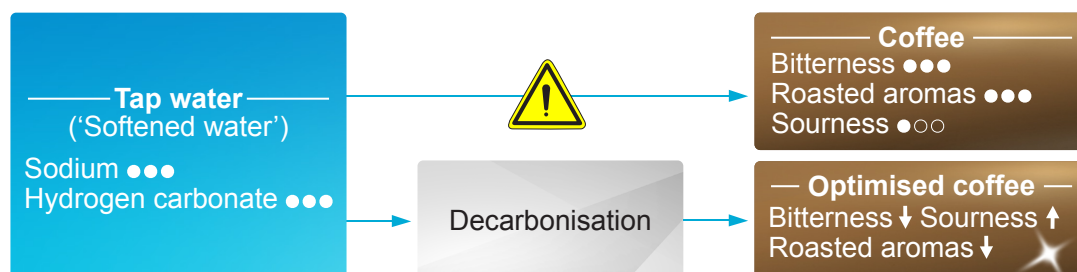
Figure 16: Too much hydrogen carbonate in the water can reduce the coffee's sourness, which has the effect of amplifying its bitterness and roasted aromas. In Southern Europe, many consumers prefer coffee that is prepared with this kind of water. In regions where this 'typically Italian' coffee taste profile is less popular, the undesirable sensory effects can be mitigated by decarbonisation.
