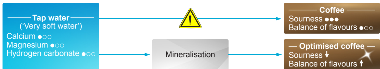
Figure 20: To prevent 'very soft water' from resulting in extremely sour coffee with an unbalanced flavour, the water can be mineralised. For this purpose, controlled amounts of calcium and/or magnesium ions together with hydrogen carbonate are released into the water to enhance the extraction of coffee flavours and to offset the coffee acids. The result is an improved balance of flavours.
