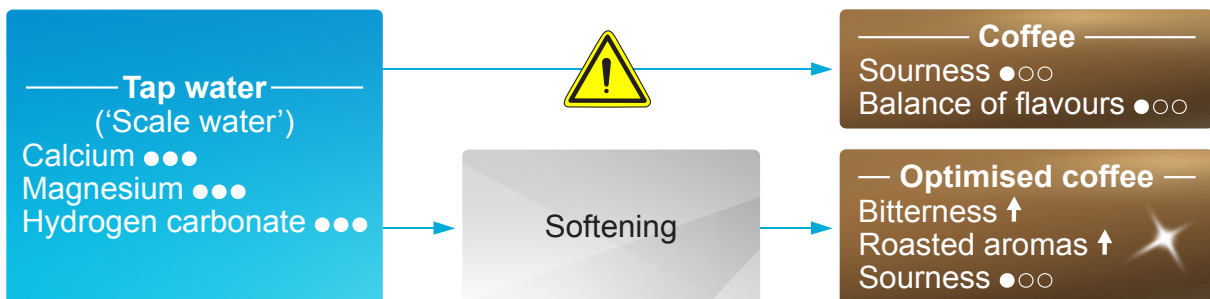
Figure 12: When dealing with ‘scale water’, a coffee flavour profile with pronounced bitterness and roasted aromas and (unchanged) low sourness can be achieved by softening.
