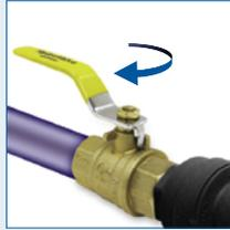
2. Shut off the water supply and collect the leaked water.
